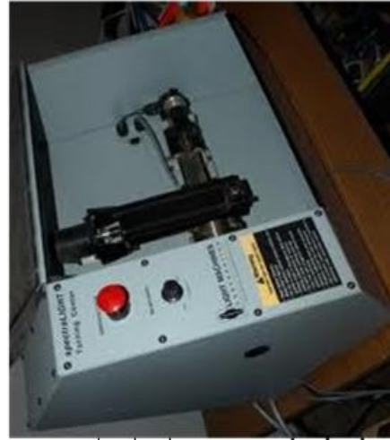
Light Machines – CNC Lathe w/auto chuck
